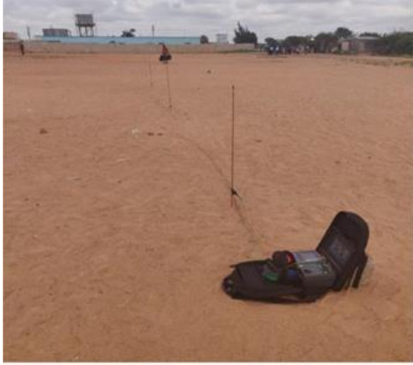
Figure 8: Soil Resistivity Testing at Kalikiliki Grounds
