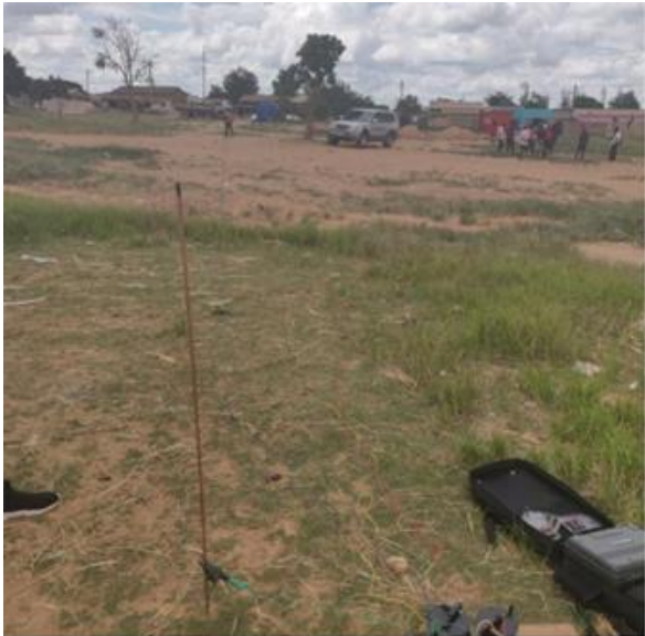
Figure 10: Soil Resistivity Testing at Kalikiliki Grounds at Kabangwe, Mtendere East
